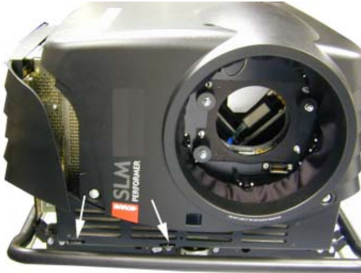
Image B-9 Dust filter bottom side
